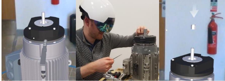
Figure 1: Left and right panels display images of a 3D virtual motor as seen through the DAQRI Smart Helmet HMD (centre panel, alongside the real physical motor). The left panel shows the work instruction for a sub-task, task step 4; requiring a user to insert a “feeler gauge” into a cavity (air gap) on the motor to measure its thickness while the right panel shows the instructions for a sub-task, task step 9, requiring a user to mount a nut on the motor shaft in order to allow them to turn it using a torque wrench.
