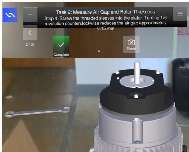
Figure 2: Shows AR text instructions (top panel) and the dynamic 3D virtual model (bottom panel) as seen through the DAQRI Smart Helmet for task step 6 “screw sleeves”.
